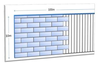
PJS robust performance boards meets and exceeds Part E B893 and HTM 2045 requirements. It can be used for walls, ceilings or floors where sound proofing is required. A 100 mm wide stud wall with PJS robust performance board gives better acoustic reduction than a 275mm block wall.
